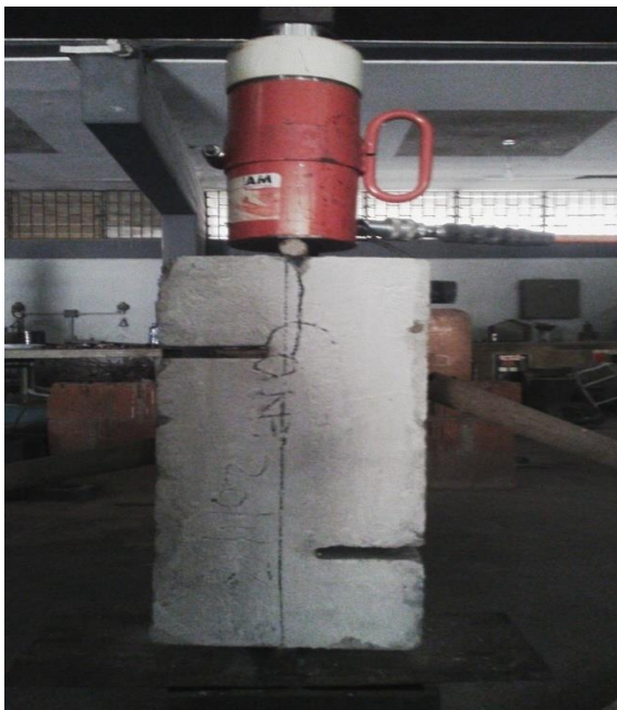
Figure 11. Shear Failure along plane of Steel Reinforced Corbel during Loading Test
