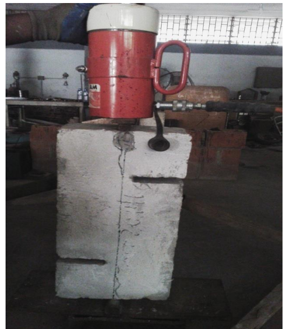
Figure 11. Shear Failure along plane of Steel Reinforced Corbel during Loading Test
